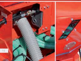
Far left: **Draining outlet** with flexible drain hose
