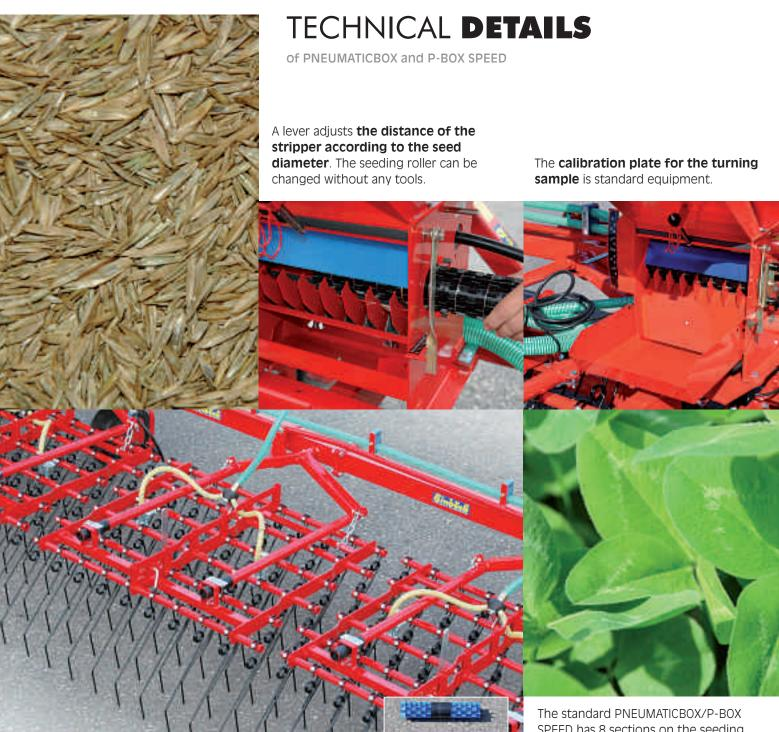
If the PNEUMATICBOX/P-BOX SPEED is mounted for example on a 9 meters Einböck GRASS-MANAGER or AEROSTAR, you need a seeding roller with 6 sections and 2 sealing plugs.
