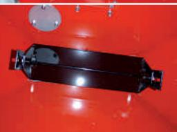
For heavy seeds we recommend the **retainer plate** mounted above the stirring shaft and the seeding roller.
