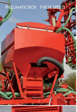
On request the PNEUMATICBOX and the P-BOX SPEED are available with a **500 litres seed tank** (with tank support and extra-large opening).
