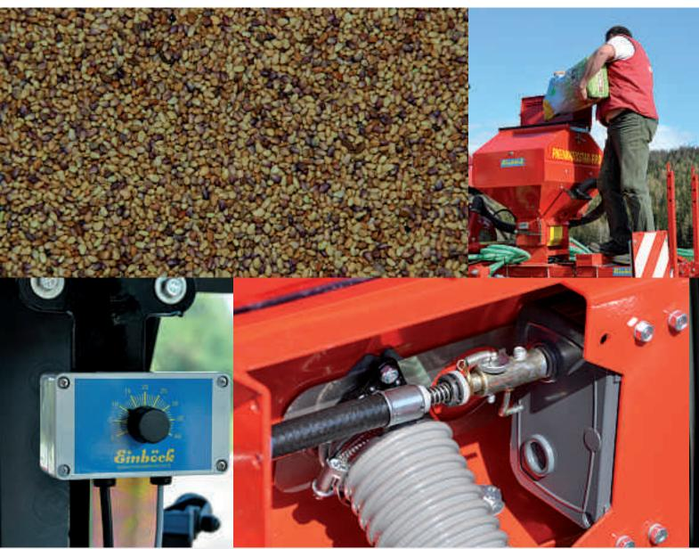
In case there are areas you do not want to seed, you can disconnect the flexible shaft from the gearbox by **taking away the bolt** where the shaft enters the gearbox.
