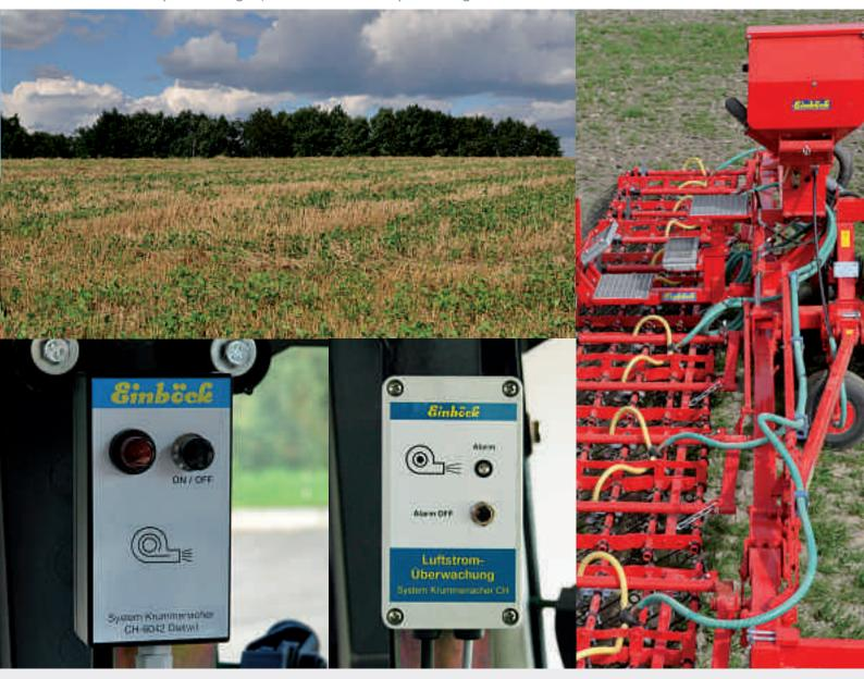
With this **control unit** you can switch on/off the electric fan.
