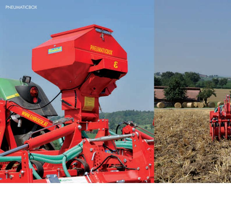
The flexible drive shaft flanged to the rubber support wheel or tail wheel transfers the power to an infinitely variable oil-immersed gearbox, which in turn powers the seeding roller and the stirring shaft by a chain drive.
